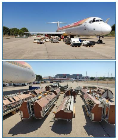
Figure 41. Aircraft going through disassembling (Envisa, 2022)
