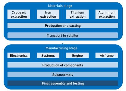
Figure 35. Diagram of the materials and manufacturing stages of the aircraft lifecycle (Adapted from Pierrat et al. 2021)
