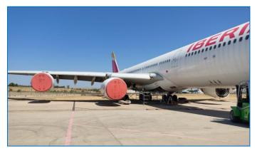
Figure 39. Aircraft put in storage with engines covered to protect them from degradation (Envisa, 2022)
