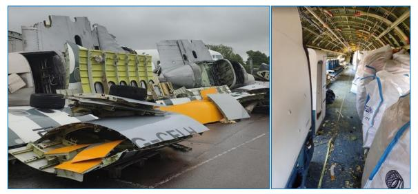
Figure 46. Dismantled aircraft sections (left) and interiors preparation for dismantling (Envisa, 2022)
